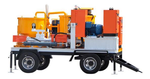
WGP400/1000/95/165DPL-E/A Grout Mixer and Pump are integrated with a screw feeder, mixing, agitator and horizontal hydraulic pump. It is mainly used to be made such as cement slurry or bentonite slurry, etc., for injecting in the sub-soil for soil consolidation, piling or even for long transport of material.
